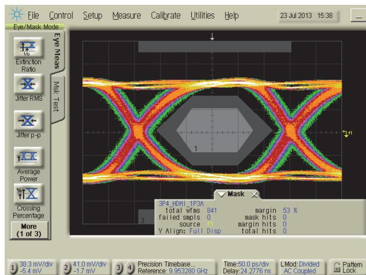
Fig 2: Example of an eye diagram showing the center mask
