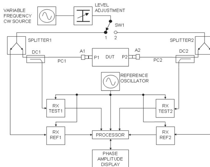
*Fig 3: The basic architecture of a two-port vector network analyser.
